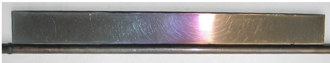
Fig. 1. The outward of the sample after its exposition to a flow of wet argon
